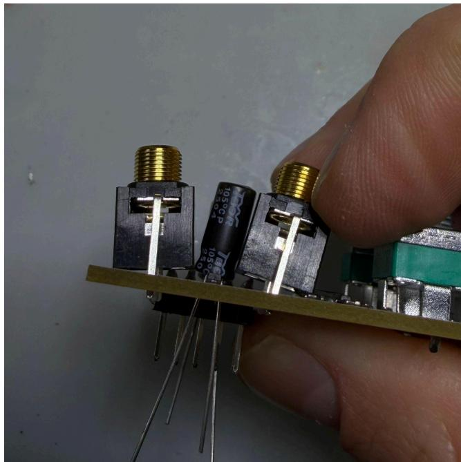
We realized that a few Sallen-Key DIY Kits were shipped with electrolytic capacitors that are slightly larger than the intended size.
