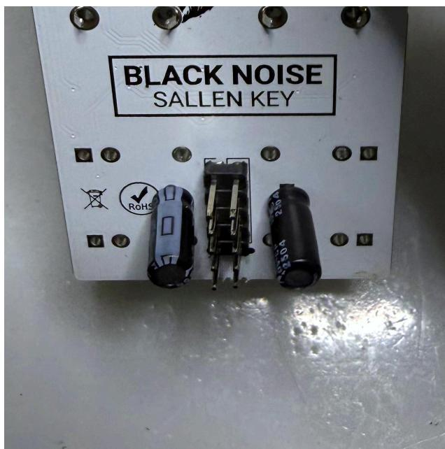
If the capacitors are too tall to be installed on the front side of the PCB, you can simply solder them on the back side instead.
